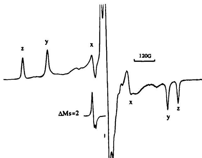
Figure 2. EPR spectrum of 3 in toluene/methyltetrahydrofuran measured in a sealed tube at 130 K.
